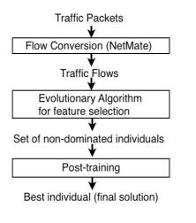
Figure. 1: System Diagram
