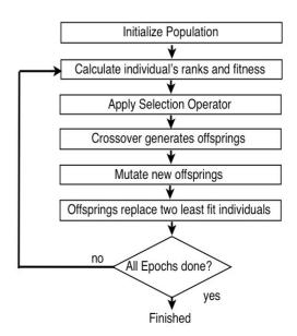
Figure. 2: Evolutionary Component Diagram
