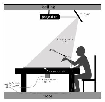
Figure 5: TractorBeam hardware configuration
