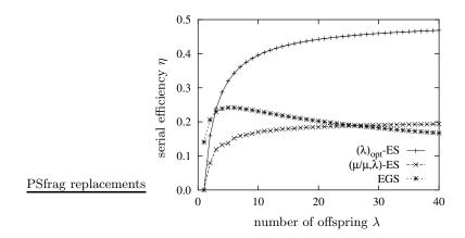
Fig. 3. Serial efficiency  $\eta$  of strategies on the sphere model in the limit  $N \to \infty$  plotted against the number of offspring  $\lambda$  generated per time step. The curves represent results for the  $(\lambda)_{opt}$ -ES described by Eq. (14), the  $(\mu/\mu, \lambda)$ -ES analyzed in [11], and EGS studied in [2].
