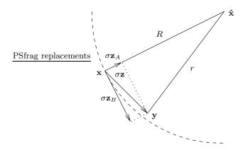
**Fig. 1.** Decomposition of a vector  $\mathbf{z}$  into central component  $\mathbf{z}_A$  and lateral component  $\mathbf{z}_B$ . Vector  $\mathbf{z}_A$  is parallel to  $\hat{\mathbf{x}} - \mathbf{x}$ , vector  $\mathbf{z}_B$  is in the hyperplane perpendicular to that. The starting and end points,  $\mathbf{x}$  and  $\mathbf{y} = \mathbf{x} + \sigma \mathbf{z}$ , of vector  $\sigma \mathbf{z}$  are at distances R and r from the optimizer  $\hat{\mathbf{x}}$ , respectively.
