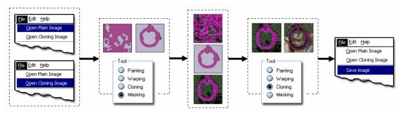
Figure 9: System workflow. 1) Open target image and cloning texture. 2) Perform self-similarity masking. 3) Rearrange cloning texture using automatic Texture-by-Numbers synthesis. 4) Clone rearranged texture onto target image. 5) Save final image.
