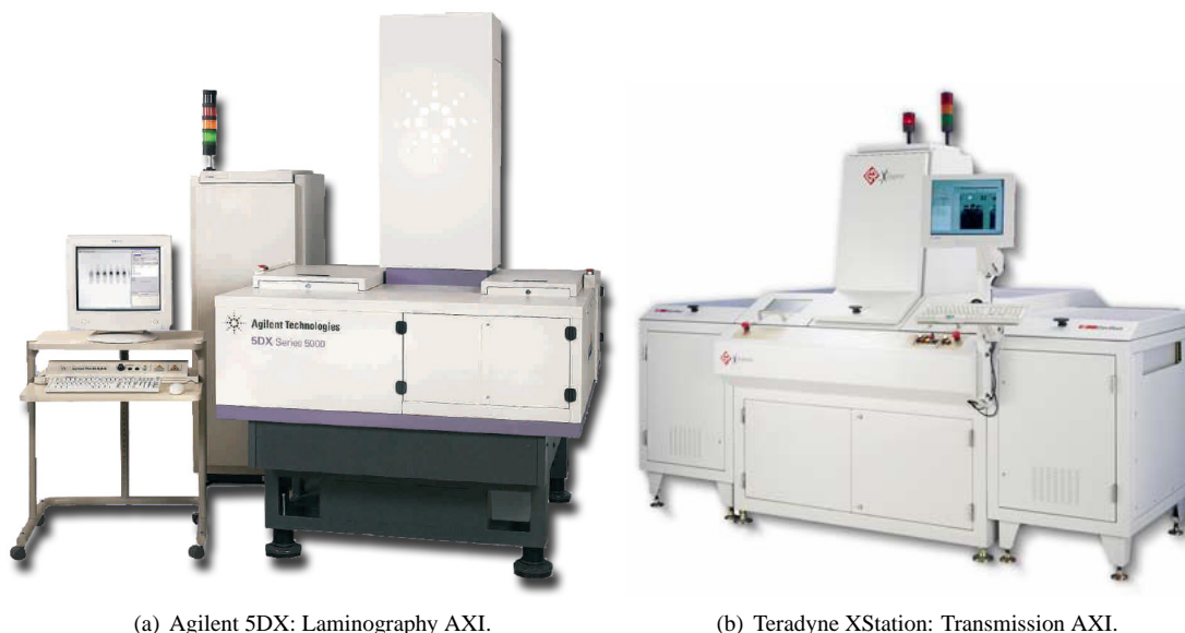
Figure 2: Two industrial machines for automated SMT testing using x-ray technology, the Agilent 5DX [1] and Teradyne XStation [14].
