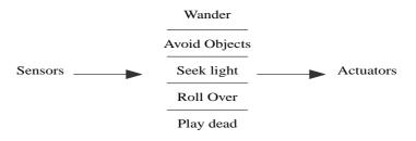
Figure 3-3. Decomposition of a mobile robot control system based on task achieving behaviours (Brooks 1986)
